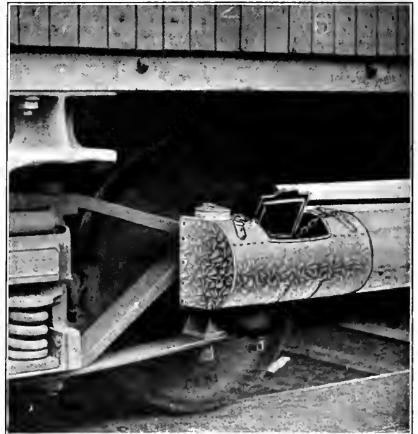
A Journal Box Cooler Which is Attached Directly to the Journal Box
